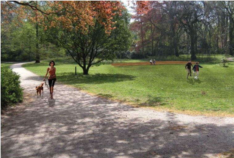
Figure 1: Illustration of the emergency flow path and the retention space in the "Ohlendorffs Park" during dry weather (left) and during extreme cloudburst events (right). Source: osp urbanelandschaften.
