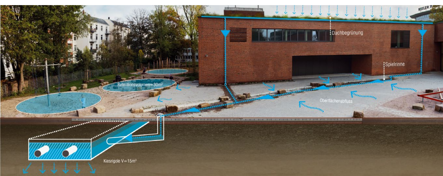
Figure 3: The water-sensitive school yard of the School Rellinger Straße with green roofs, swales, infiltration structures and a drainage channel.
