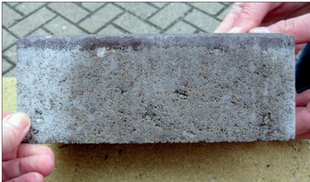
Bottom: Iron sludge for paving stone
